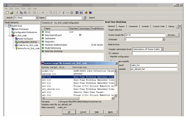
Change the code generator to Real-Time Workshop® Embedded Coder™ software
